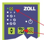
Point Remote Controller at unit and press view/enter button again. Green light on Remote Controller will show Manual Scenario Mode is selected.
